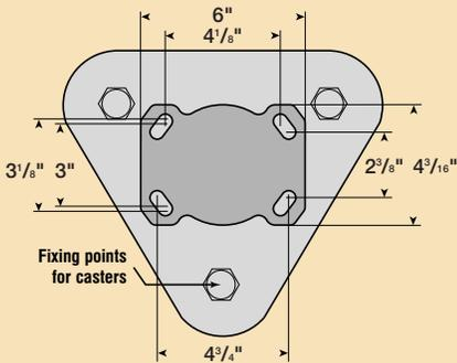
When fitting at 4-3/4" x 2-3/8" hole centers, use 1/2" diameter bolts.
